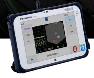
The XaverNet<sup>TM</sup> system is a remote wireless ToughPad that works in combination with Xaver<sup>™</sup> 100 and Xaver<sup>™</sup> 400 systems. It enables the user to receive real time visual data and fully control remotely up to four Xaver systems simultaneously.
