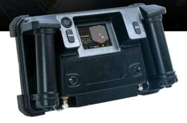
The Xaver<sup>TM</sup> 400 is a compact Radar based device, optimized for quick tactical decision making in urban operations. It provides real-time mission-critical information on live and static objects hidden behind walls and barriers, including:
